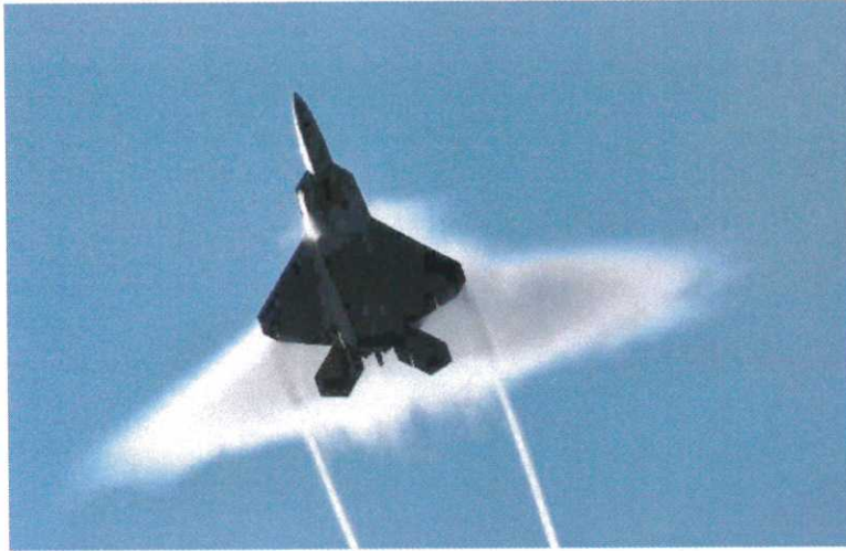
A U.S. Air Force F-22 'Raptor' executes a supersonic flyby at low altitude, producing pronounced wingtip vortices and a 'shock egg'. 3
