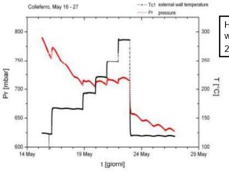
Hydrogen loading increased when temperature was below 200 degrees C
