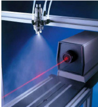
Figure 8.1: Malvern Analyzer (Malvern 2600) which is a laser measurement device for droplet size measurement, the picture shows a spray from effervescent atomization nozzle and the measurement device [32]
