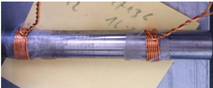
Figure 3. Coler replica magnet with driving coil (right) and pick-up coil (left) to study the magneto-acoustic resonance
